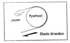
Use a strip of scrap paper and slide it between the blade and the flywheel while it is running.
