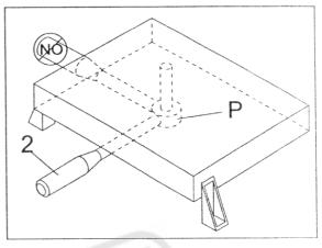
To move the vise in either direction, the vise jaw must be unlocked at two points.
