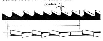
This type of blade is the most suitable for the cutting of section bars and large and thick pipes as well as for the cutting of solid bars at maximum machine capacity. Available pitches: 3-4/4-6.
